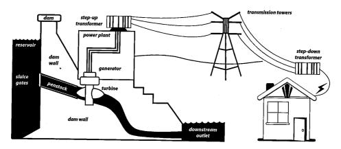
The principle of electromagnetism is used to generate electricity. Just as a current in a wire generates a magnetic field around itself, so a moving magnetic field generates a current. Inside the generator, a magnet spinning inside a coil of copper wires generates a current in the coil—electricity!
