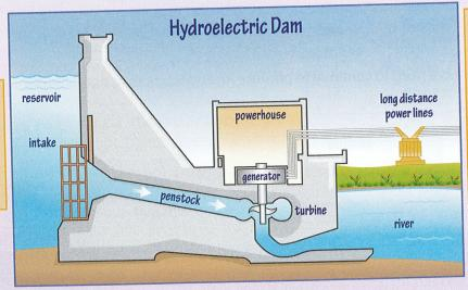
The flowing water pushes the blades on the propellerlike turbine, which turns a metal shaft connected to the electric generator. This machine transforms mechanical energy into electricity.
