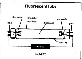
A fluorescent light globe is a sealed glass tube filled with argon and containing a small amount of mercury, a poisonous metal that is a liquid at room temperature. The glass tube can be a long strip, circular or coiled to fit in standard lamp fittings.
