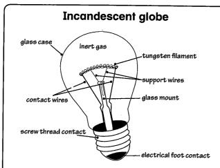
The components of an incandescent globe are housed in a sealed glass case containing a gas called argon. The metal filament coil is about 2.5 cm long. It is made from two metres of extremely thin tungsten wire. To fit into the space, the fine strip of wire is wound into a tight coil which is then wound around itself to make an even tighter coil.
